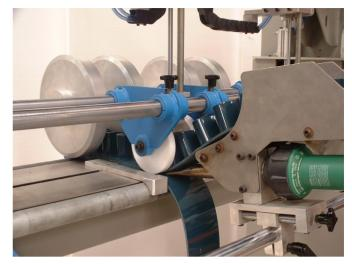
The hot air welders are easily regulated, as the profile can be attached using cold vulcanisation, thanks to the two positions for these welders.
